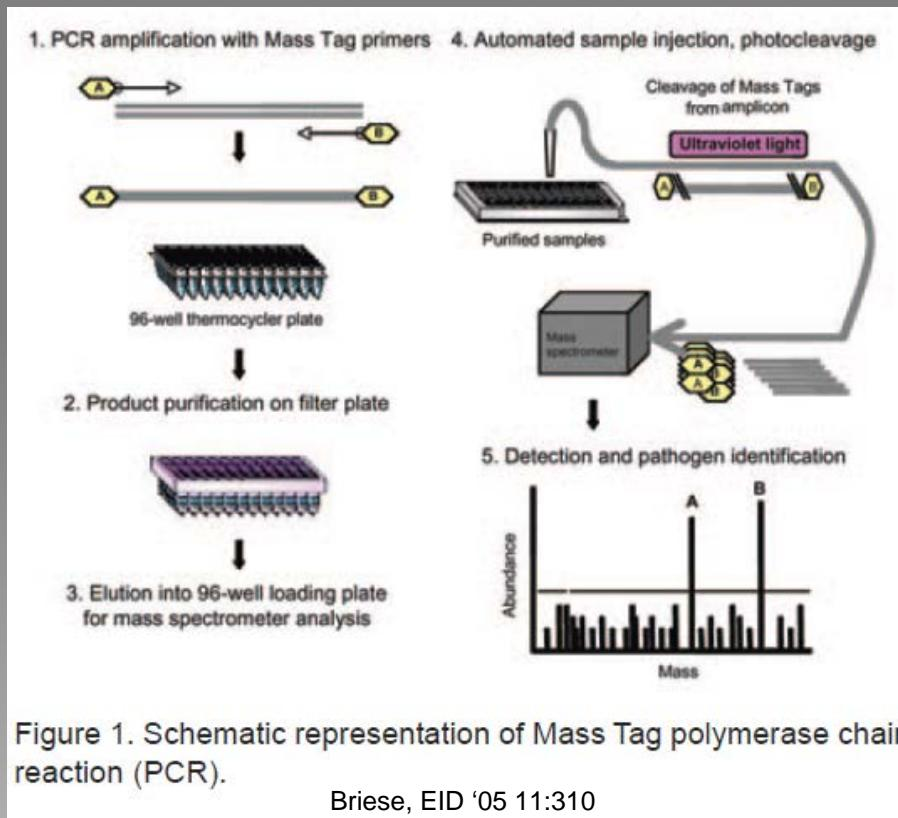
Figure 1. Schematic representation of Mass Tag polymerase chain reaction (PCR).
